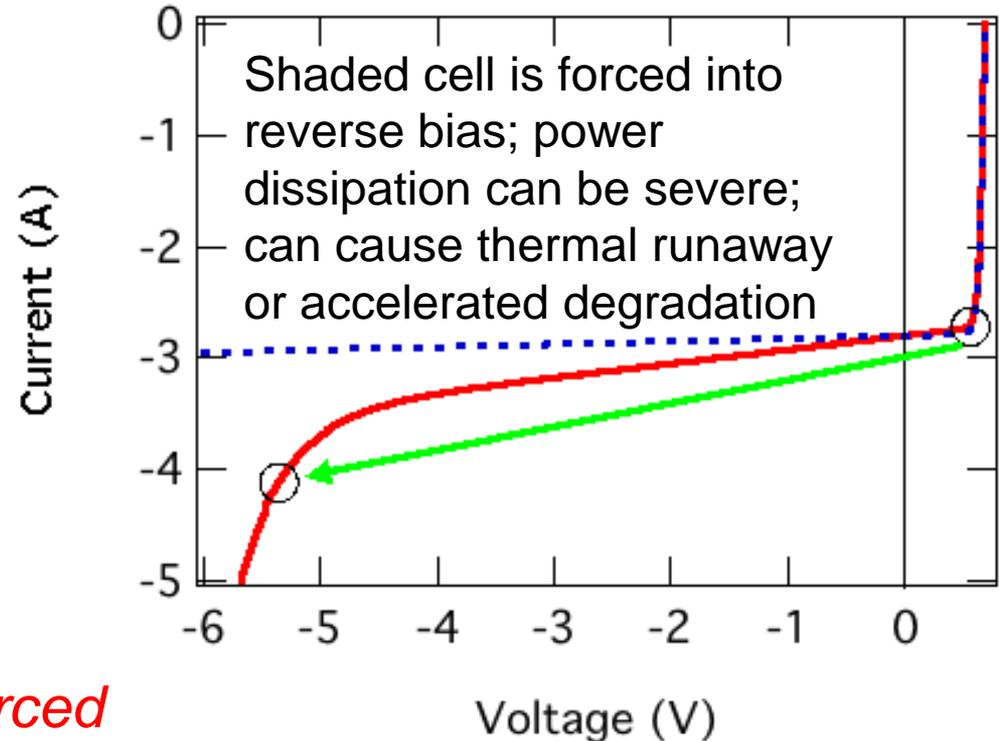
“Hot-spot test” is part of qual test
