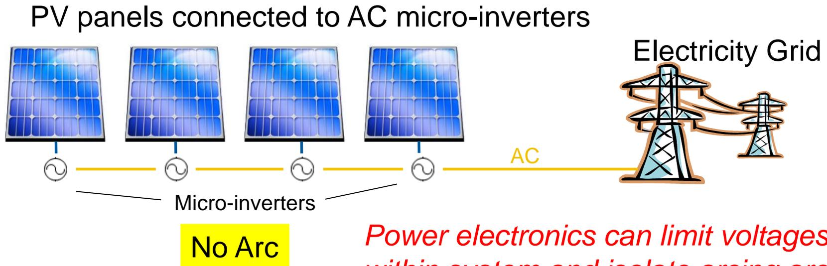
*Power electronics can limit voltages within system and isolate arcing areas*
