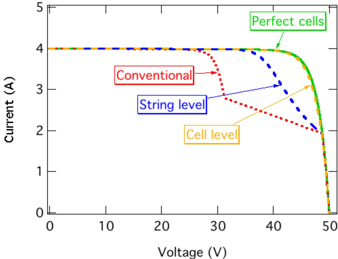
Simulation of 50% loss of current from 1 cell; power electronics 100% efficient; Three strings of 24 cells each, only one string has bad cell.
