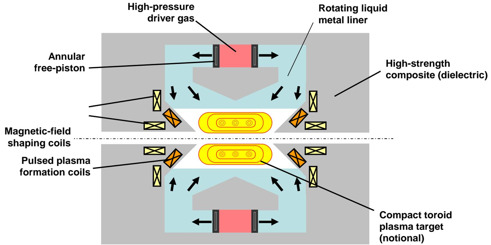
**The same arrangement would be used for laboratory experiments, including scientific breakeven, adjusting the size, liner material and plasma conditions. Note that the pneumatic energy storage/pulsed power subsystem is contained within the device, but could be replaced by a high-field, theta-pinch coil (as in early NRL experiments).**
