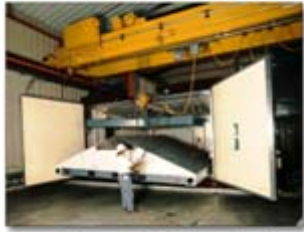
The only large-scale, 3-D climate simulator (for attic systems, etc.) in the U.S.
